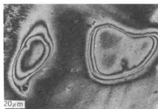
Fig.6 Closed inversion walls of an oriented film of Z-6 of frozen mesophase annealed at 190\text{ }^{\circ}\text{C} for 10min
