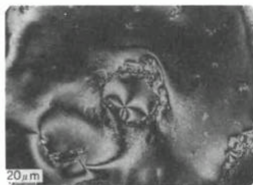
Fig.5 POM micrograph of schlieren texture with 6 brushes in the nematic phase of Z-6
